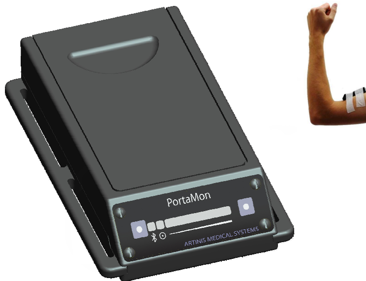
Portable NIRS device: The PortaMon
